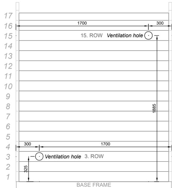
6.2 Cover the openings with ventilation grids or valves, as shown in Scheme 6.2. Use 3.5x40 black screws for fixing.
